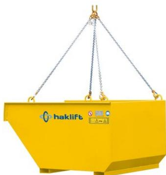
The liftable self dumping bin is a practical and durable tool for handling construction waste. The container is equipped with four lifting points, ensuring stability during lifting. The container can be tipped when the front legs of the lifting chain sling are detached from the lifting points. It is suitable for handling various construction materials, such as sand, gravel, demolition waste, and other loose materials. The container can also be used with a forklift.
